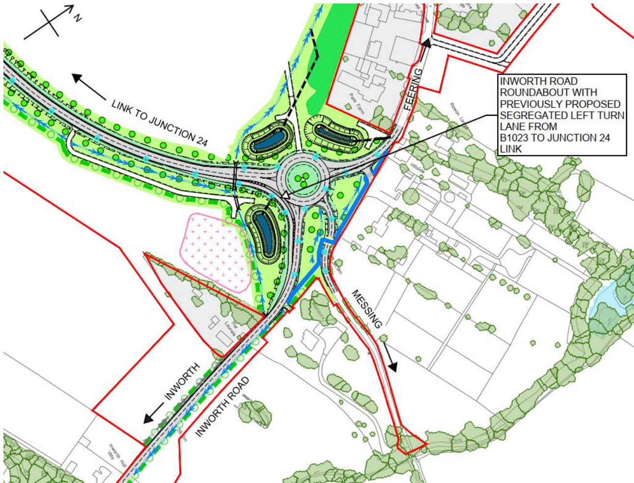
Plate 1.1 Inworth Road Roundabout with Segregated Left Turn Lane as submitted for DCO Application
